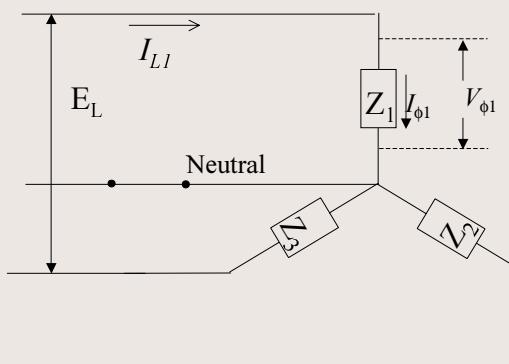
$$V_\phi = E_\phi, \quad I_{\phi l} = I_{Ll} = \frac{V_{\phi l}}{Z_l}, \quad I_N = I_{\phi l} + I_{\phi 2} + I_{\phi 3}$$
