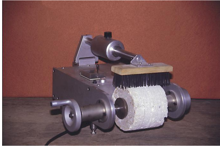
Figure 1. Mechanical wet/dry brushing device
