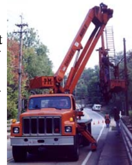
A snooper. This truck allows you to get up under bridges.
