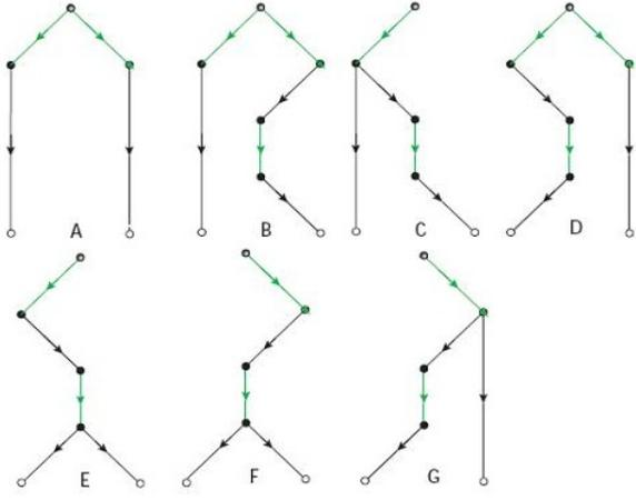
Fig. 5. Multicast routes in singular-Symmetric Butterfly network
