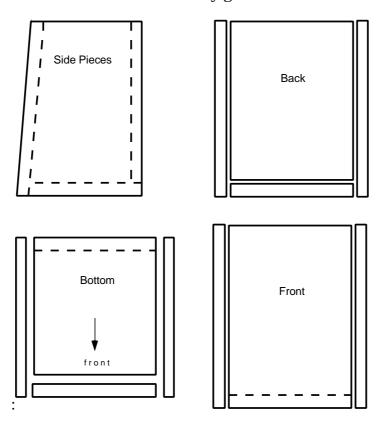
From the guide, you can see that the side panels are supposed to go on top of everything else, while the back panel is surrounded by glass on all four sides.
