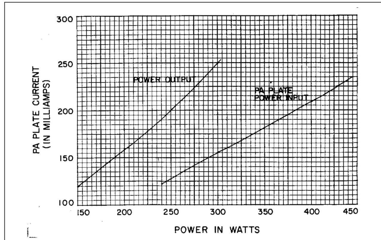
Figure 1 - Power and PA Plate Current Levels
