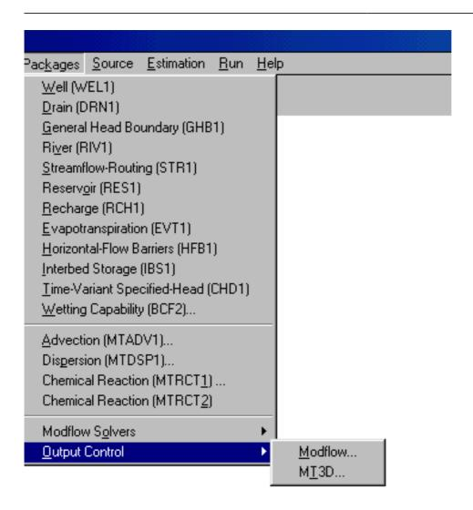
The data parameter input options are shown below for Visual MODFLOW. The example on the screen is the Lowgan model prepared by NGRI and sent to the Consultant as an attachment to e-mail. This example was also used in the Workshop. The aquifer modelled is the Ganga-Kali interstream area, an alluvial aquifer heavily exploited by drilled wells. The input parameters that describe an aquifer system are as follows:
