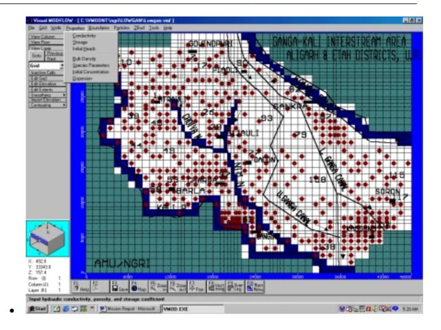
Processing Modflow input parameter data screen looks as shown below. Both screens (Processing Modflow and Visual Modflow) indicate the need for various categories of data to be collected and prepared for the model. Much of the model input should come from a GWIS to be established using the GWW package or some other software.
