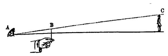
655. A is the eye, B is the hand extended to the full length of the arm, and holding the instrument to be graduated, C is a man of medium height.
