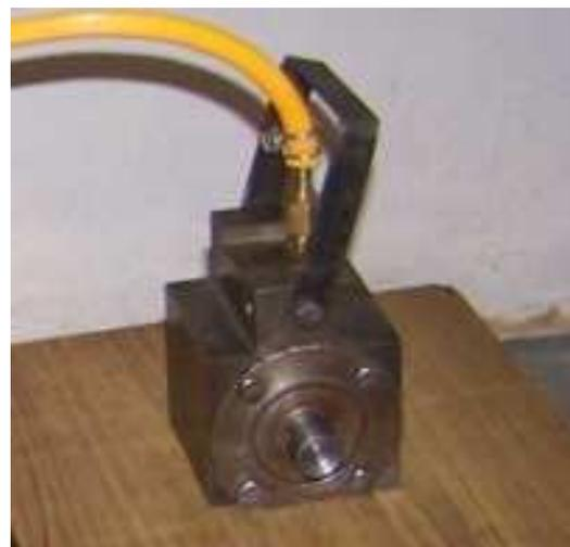
Fig. 3 Compressed Air Turbine-Working Model
