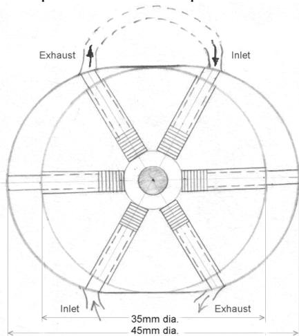
**Fig.5** Dual inlet & exhaust Air Turbine Model
