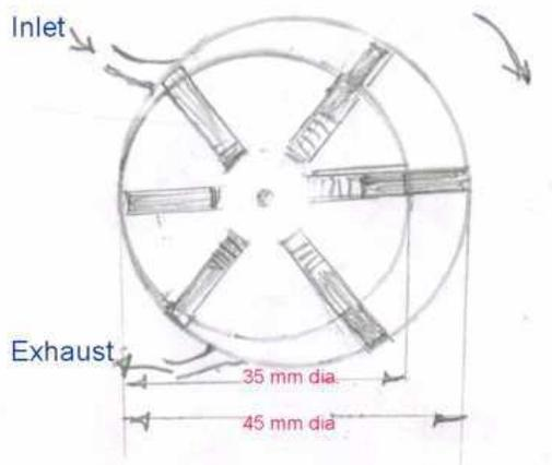
Fig. 1 Compressed Air Turbine –Concept & Cycle
