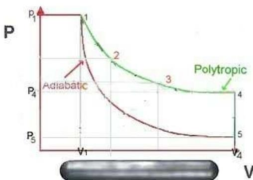
Fig.2 Isentropic cycle for Air Turbine
