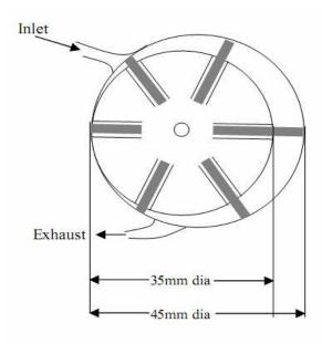
$$w = n \left(\frac{\gamma}{\gamma - 1}\right) p_1 v_1 \left\{ \left(\frac{p_4}{p_1}\right)^{\frac{\gamma - 1}{\gamma}} - 1 \right\} - n \left(p_4 - p_5\right) v_4$$
