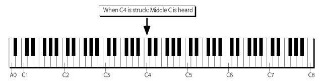
Each semitone is represented by a MIDI note name. The octaves—which begin at each C natural—are numbered, as shown above. The ASR-X Pro can address MIDI notes from A0 to C8.
