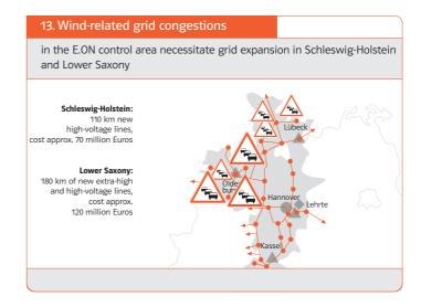
In both cases, the plans are based on pure onshore expansion scenarios. If offshore wind parks will also be built on a greater scale in the future, additional grid expansion measures would also be necessary in the extra-high voltage grid.
