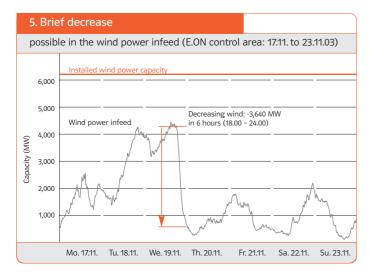
FIGURE 4 shows an example of the wind power infeed pattern in the E.ON territory during a week with strong winds. The difference between minimum and maximum infeed in this example was over 4,300 MW – equivalent to the capacity of six to eight large coal-fired power station blocks.
