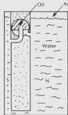
Fig. 7. Small oil valve with central vertical tube. Drawing not to scale.
