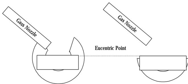
Figure 1: The left is used by Morris, S. et al. and the right is used in this work. The right can prevent the gas nozzle hitting the sample but the left.
