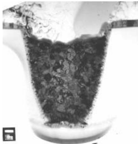
Figure 10: XTEM micrograph of CVD W-plug. The complete plug structure was preserved and grain was observable.
