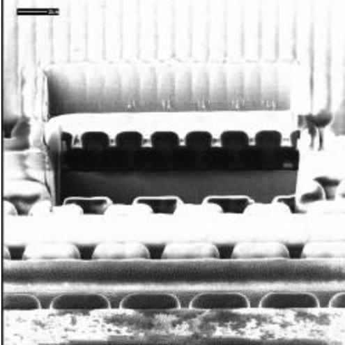
Figure 5: FIB cross-sectional micrograph of selective area before sacrificial metal film coating.
