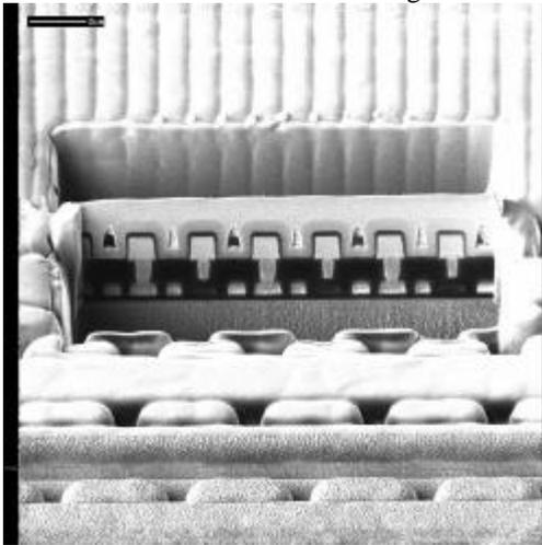
Figure 6: FIB cross-sectional micrograph of selective area after sacrificial metal film coating. The charging effect was minimized and the fine milling could be performed without suffering charging effect induced beam shifting.
