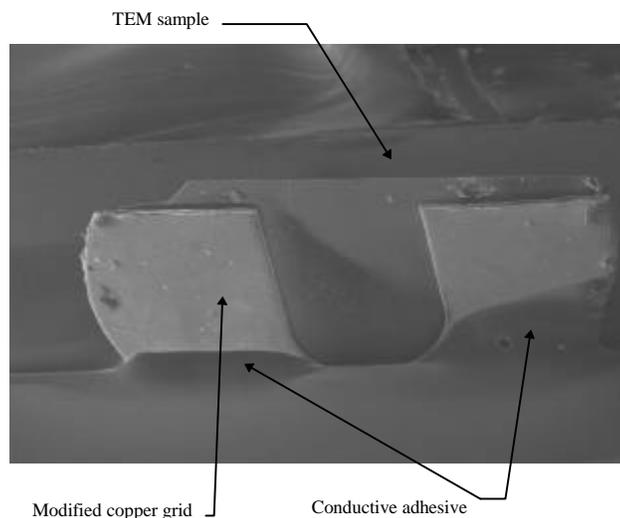
Figure 2: SEM micrograph of TEM sample mounted on the modified copper grid.
