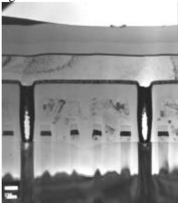
Figure 7: XTEM micrograph of CVD W-plug with high aspect ratio (6:1). The streaking or masked effect was obviously observed.
