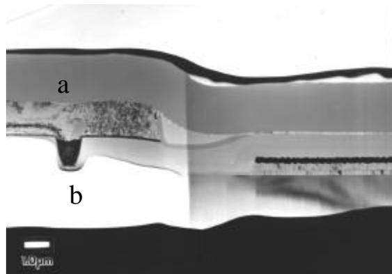
Figure 9: XTEM micrograph of CVD W-plug. By using two axes tilting and selective area etching, hole due to melting of materials under the Al line is clearly visible.
