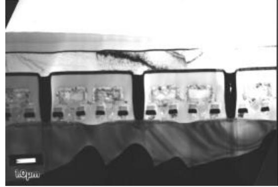
Figure 8: XTEM micrograph of CVD W-plug with high aspect ratio (6:1). The streaking or masked effect was almost eliminated.
