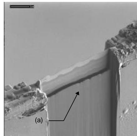
Figure 3: Scanning ion micrograph of XTEM membrane fabricated by FIB. (a) With the aid of Halogen gas assisted etching, the streaking / masked effect induced by IBICE can be obviously observed.
