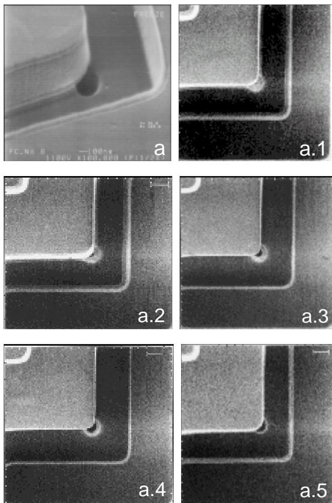
**Fig.1:** (a) An example of severe W plug loss after solvent stripping. (a.1)~(a.5) The extent of W plug loss divided into 5 levels from plug loss level 1 to 5.
