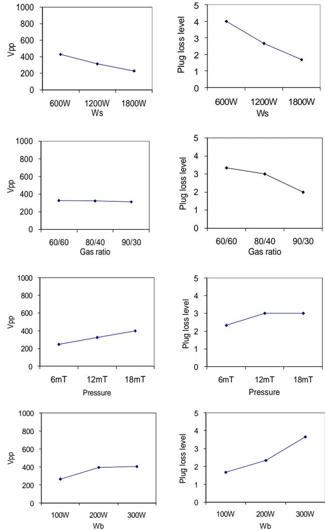
**Fig.2:** Individual etch parameter (Ws, gas ratio, pressure and Wb) effects on plasma potential and W plug loss.
