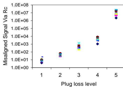
**Fig.3:** Electrical test result shows misaligned via resistance as a function of plug loss level.
