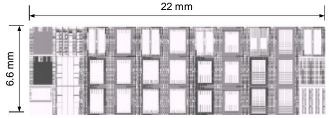
**Fig. 4:** Layout of four types of addressable failure site and PCM test structures.
