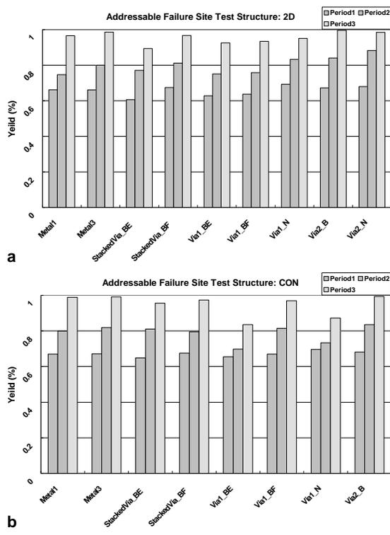
Fig. 7: The yield trends test structure categorized by test key module. (a) 2-D type. (b) CON type.
