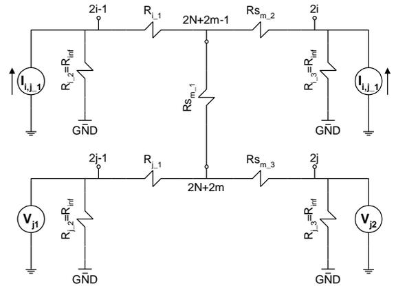
**Fig. 5:** Schematic graph of short-circuit model.
