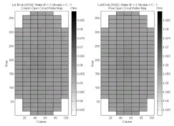
Fig. 9: L. Wafer map of Column direction M3 sheet resistance. R. Wafer map of Row direction M3 sheet resistance.
