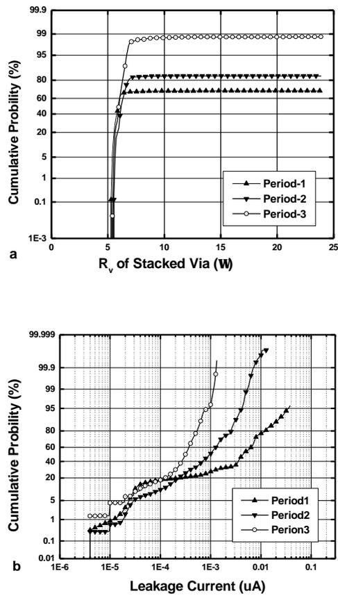
Fig. 8: The effect of process optimization. Stacked borderless via test structures is used as optimization index.
