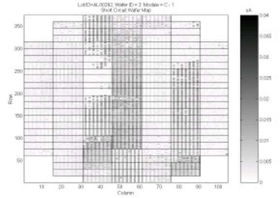
Fig. 11: Wafer map of leakage current. Normal process.
