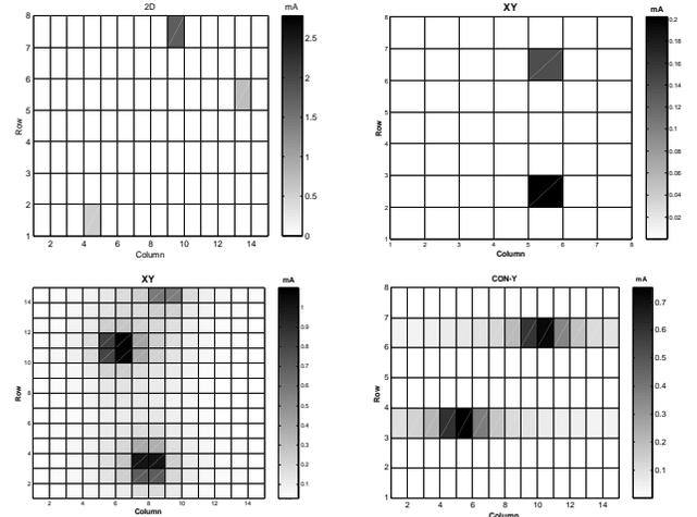
**Fig. 6:** Leakage chip map of four types of test structure. (a~d) are 2D, XY, CON, and CON-Y, respectively.
