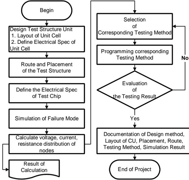
**Fig. 2:** The flow shows the development methodology of the novel test structure.
