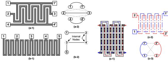
**Fig. 1:** Typical test structure and their geometry graphs. The solid line represents the conductive component and the dash line stands the possible leakage paths. (a-1), (b-1) Schematic layout of conductive layer. (a-2), (b-2) Geometry graph. (c-1) Schematic layout of Contact/Via chain. (c-2) Placement and routing. (c-3) Geometry graph.
