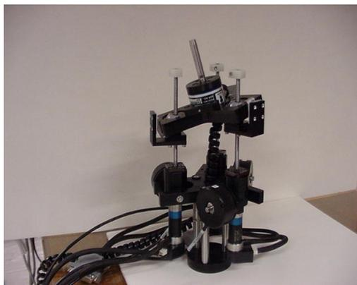
Figure 4. 3-DOF in-parallel actuated manipulator
