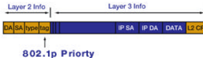
Figure 4. IEEE 802.1p adds three priority bits (tag) to the Layer 2 header.
