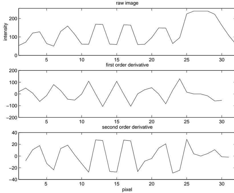
Figure 7.3: Edge Detection on an image of the goal and ball (far right)
