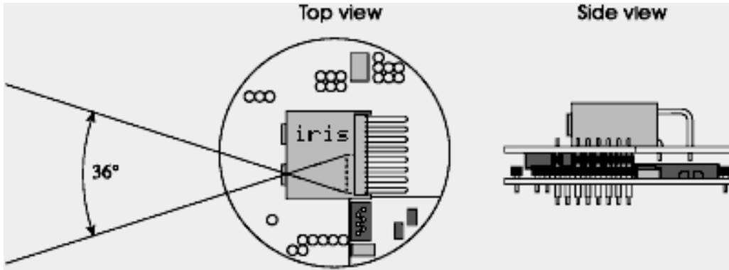
Figure 4.2: Schematic of the K213 vision turret
