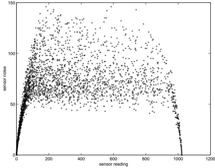
Figure 5.1: Scatter plot of IR sensor noise as a function of sensor value for data collected
