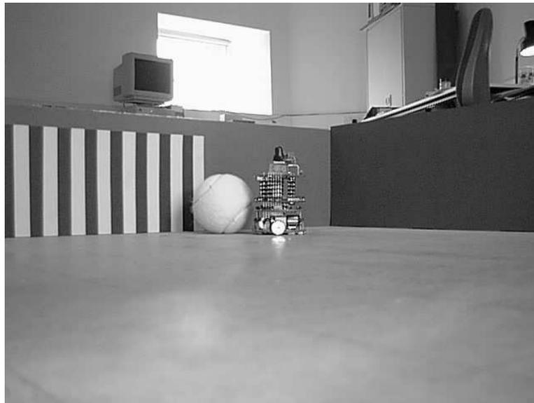
The task was inspired by robot football. The use of ‘football’ to describe the behaviour is perhaps hyperbolic; more prosaically it is pushing an object to a target. In terms of behavioural complexity in evolutionary robotics this task is state of the art. The task and environment were shaped by the
