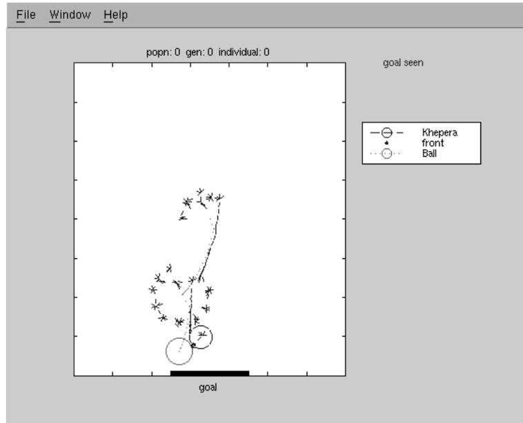
Figure 8.10: Hierarchical goal scoring behaviour — spiraling to align ball, goal and Khepera, then pushing to goal.
