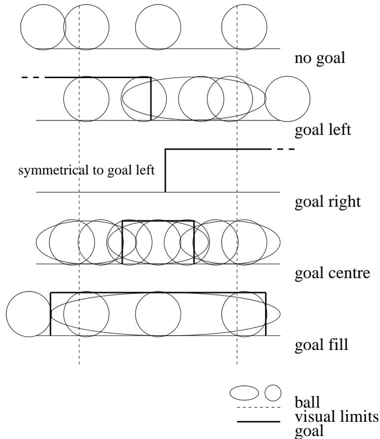
Figure 6.1: Classes of image with respect to overlapping edges of ball and goal and visual limits
