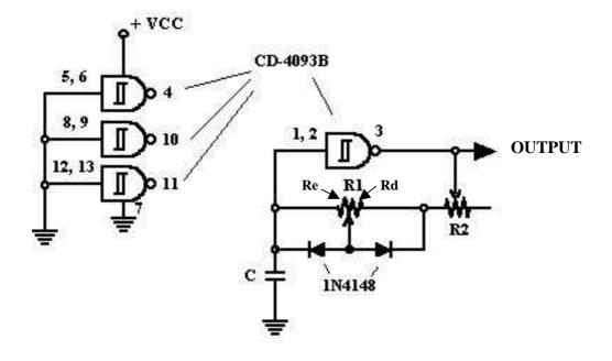
The symmetry is controlled by R1 The frequency is controlled by R2
