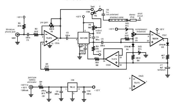
The signal is pre-amplified by the TL074 first section (CI1A) and excites the MC1350 (CI2) that has two outputs: one, with DC isolation, that is the signal final output and another one that is amplifies by a TL074 section (CI1C) with open mesh, that is, with maximum gain. The output of this section is half-wave rectified by D2 (there was not the need of full-wave rectification) and filtered by resistor R7 and the tantalum (for less loss) capacitor C7.
