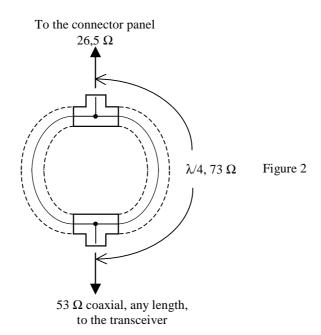
A piece of 53 Ohm coaxial with length **2L** (any) is connected between the two antennæ in such a manner that it comes from one antenna, passes through the shack and returns to the other antenna as in figure 1.
