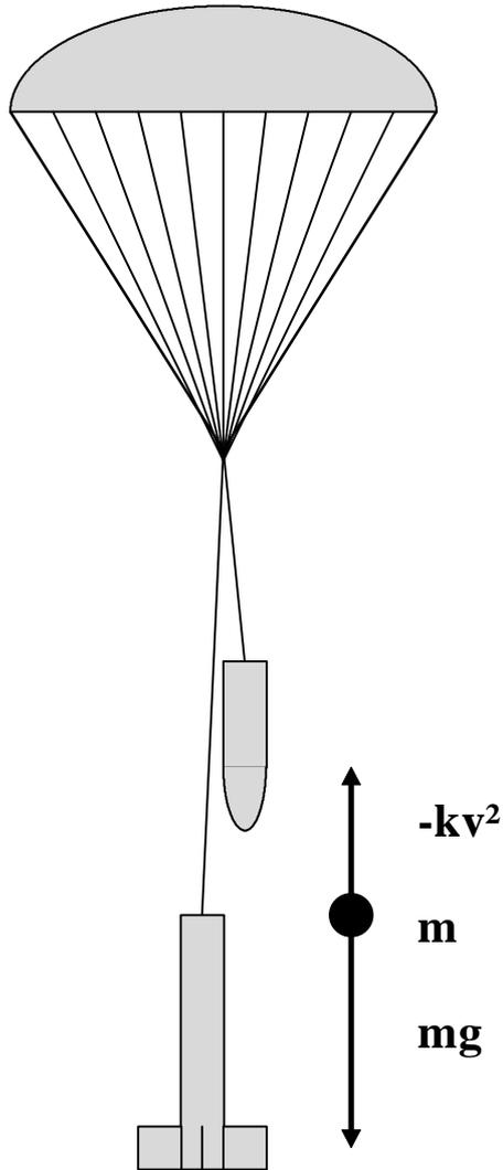
Fig. 3 Forces acting on a rocket travelling vertically downward in a parachute
