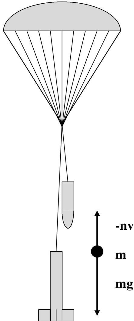
Fig. 4 Forces acting on a rocket travelling vertically downward in a parachute
