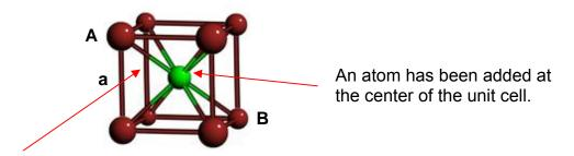
The line joining opposite corners of the cube (AB) and passing through the central atom is called the body diagonal.
