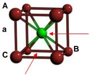
The diagonal is drawn from A (upper left corner on the front face) to B (lower right hand corner on the back face) passing through central atom and is the hypotenuse of the triangle ACB.
