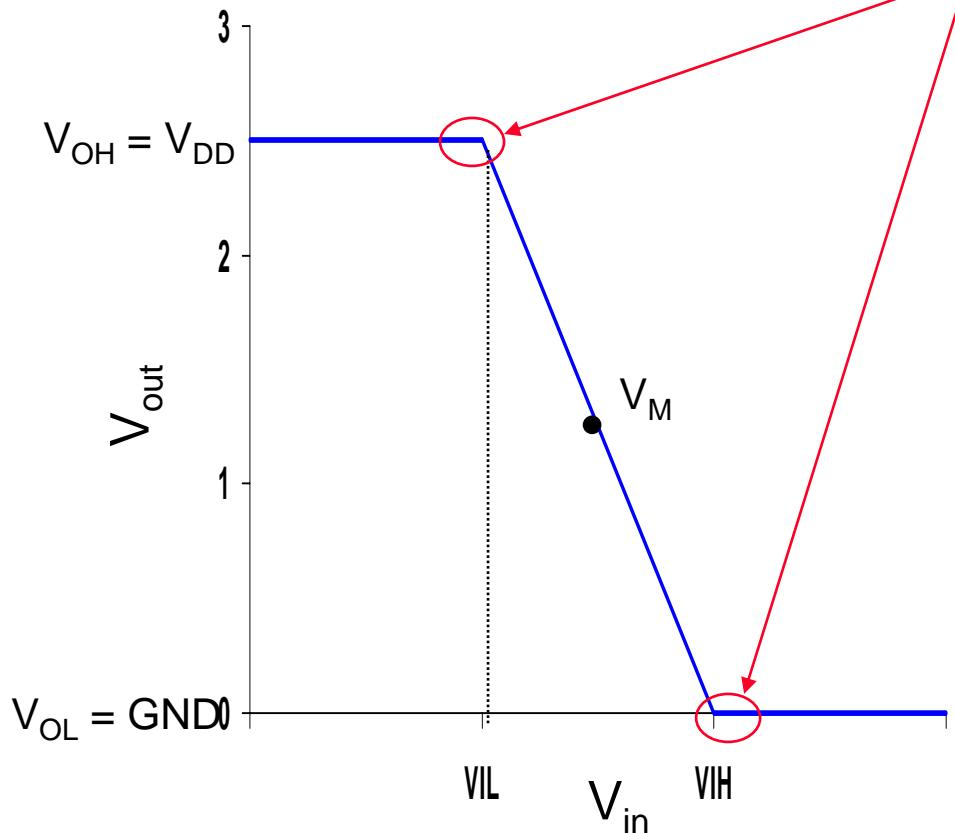
By definition,  $V_{IH}$  and  $V_{IL}$  are where  $dV_{out}/dV_{in} = -1$  (= gain)
