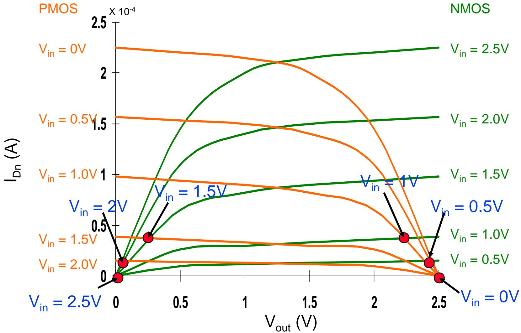
0.25um,  $W/L_n = 1.5$ ,  $W/L_p = 4.5$ ,  $V_{DD} = 2.5V$ ,  $V_{Tn} = 0.4V$ ,  $V_{Tp} = -0.4V$
