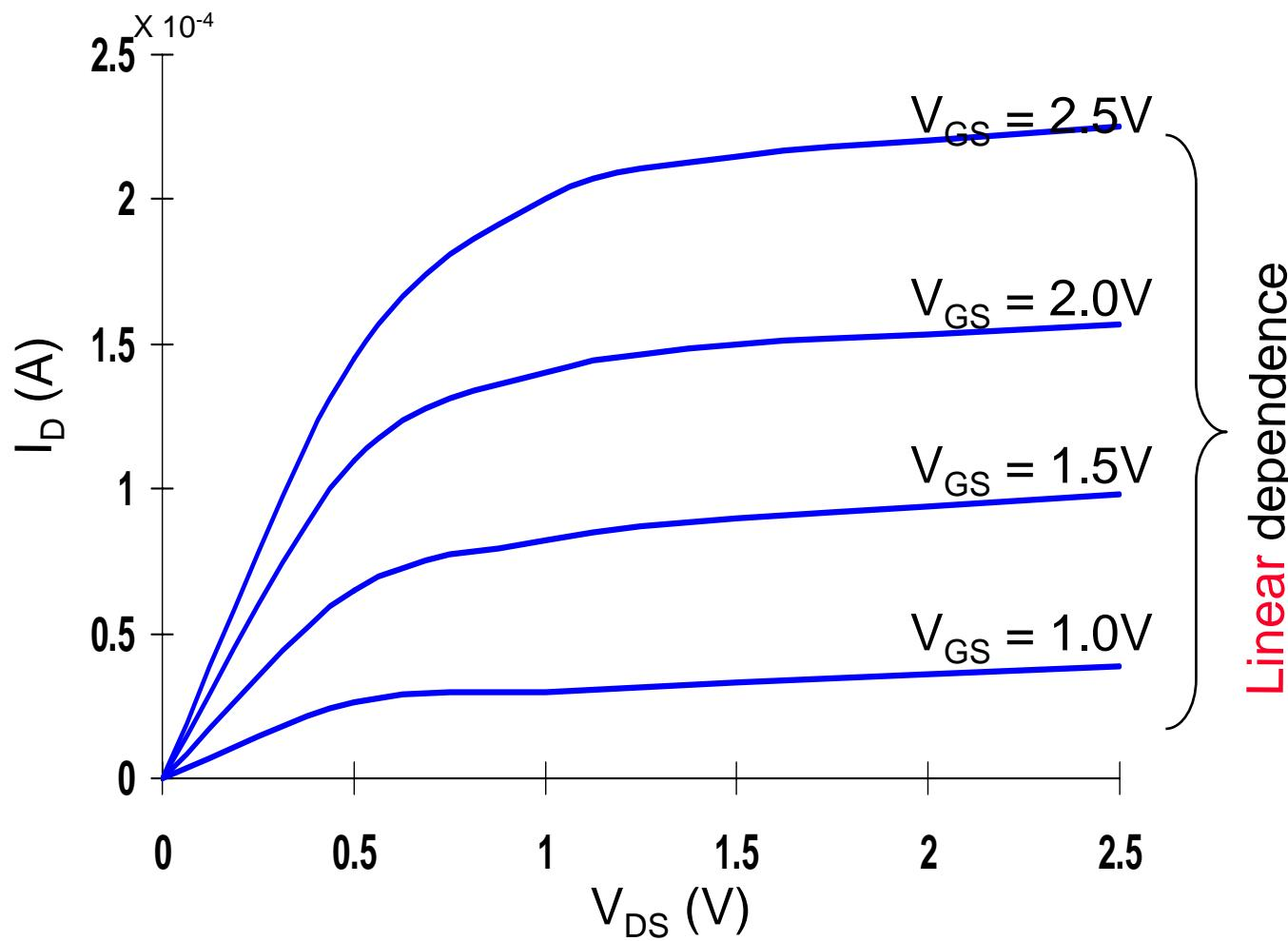
NMOS transistor,  $0.25\mu m$ ,  $L_d = 0.25\mu m$ ,  $W/L = 1.5$ ,  $V_{DD} = 2.5V$ ,  $V_T = 0.4V$
