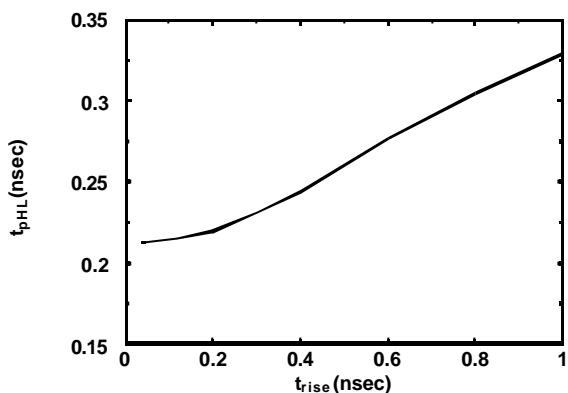
$$t_{pHL} = \sqrt{t_{pHL(\text{step})}^2 + (t_r/2)^2}$$
