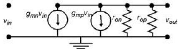
$$g = \frac{v_{out}}{v_{in}} = -(g_{mn} + g_{mp}) \times (r_{on} \parallel r_{op}) = -1$$
