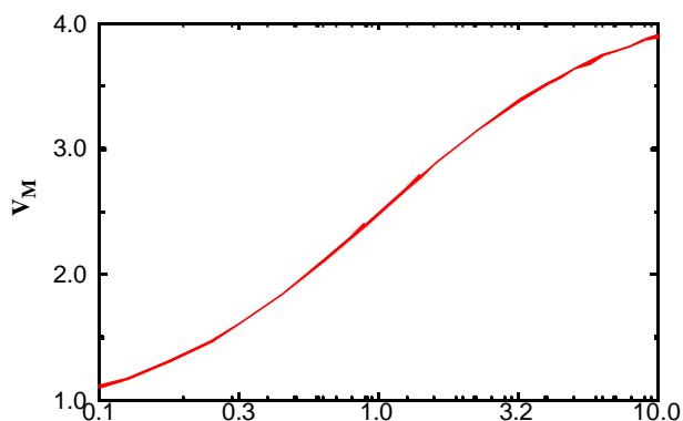
$$V_M = \frac{r(V_{DD} - |V_{Tp}|) + V_{Th}}{1+r} \quad \text{with} \quad r = \sqrt{\frac{k_p}{k_n}}$$
