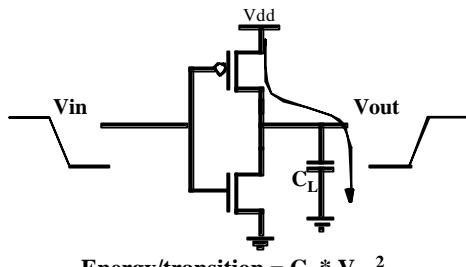
$$\text{Energy/transition} = C_L * V_{dd}^2$$
