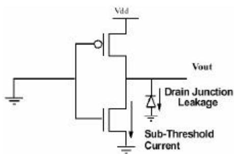
Sub-threshold current is one of the most Compelling issues in low-energy design
